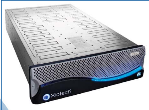
Fig. 2. ISE-based Emprise 5000 can be used as direct- or switch-attached storage, part of a NAS solution, or the foundation of an Emprise 7000 SAN system.
